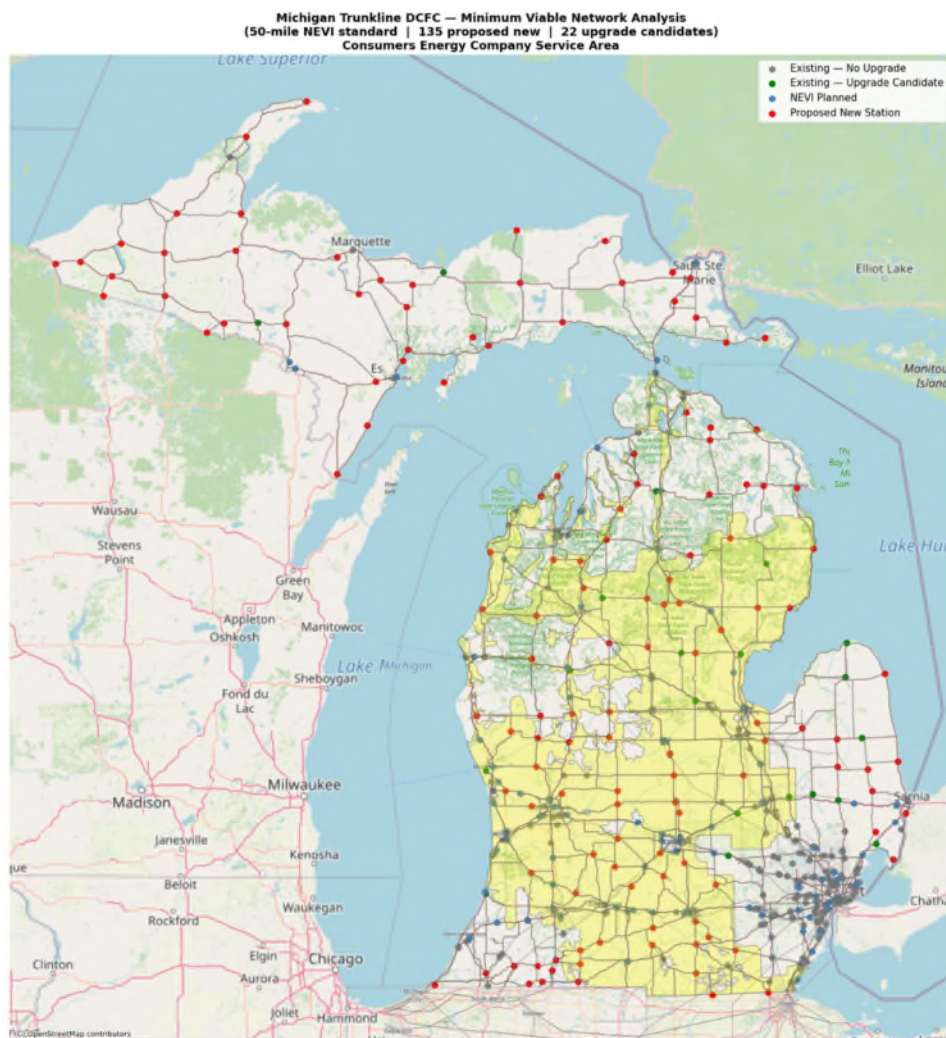
Figure 1: MDOT trunklines, existing and planned DCFC stations, and gaps relative to a Michigan Minimum Viable Network. Consumers' service territory is highlighted, showing 10 gaps.
